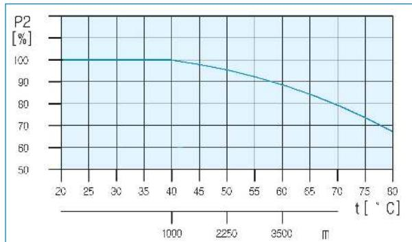
Example) When the pump should be installed sea level 3500m and ambient temperature 60C, The performance ability drops 80%.
