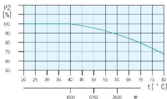
Example) When the pump should be installed sea level 3500m and ambient temperature 60C, The performance ability drops 80%.
