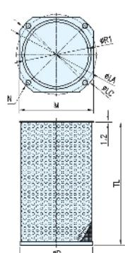
● Material 재질 : Steel (SB41), Finishing 도금 : Plating of Black (흑착색), 12Mesh : F, HF, HMFS, HMFD, MF, BMF
